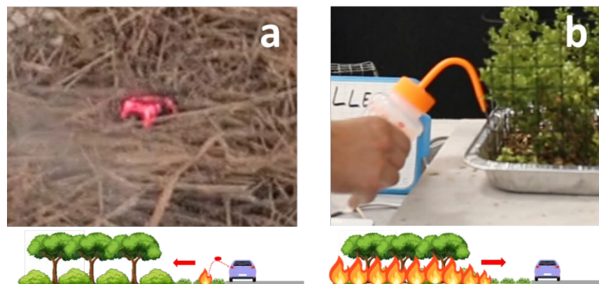
Figure 7 : The 2 ignition protocols : the glowing brand (a), and the alcohol line (b).
