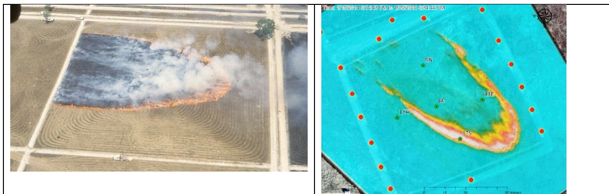
Figure 11: Fire footprints from the experiments used here. Visible image, taken from a helicopter during the AU grassland fire experiment C064, on the left. Infrared image taken from a fixed wind UAV during the Camp Swift burn block 1 experiment, on the right.
