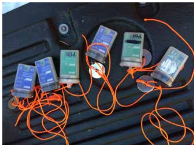
Temperature sensors ready to be deployed to measure snow presence by recording ground temperature.
