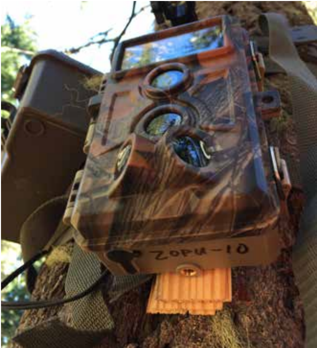
Timelapse camera deployed in a tree to measure snow depth at a three-hour timestep.
