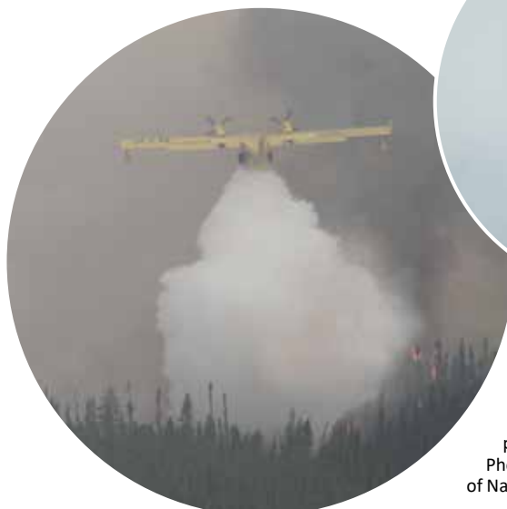
A CL-415 dropping along the fire's edge, ensuring safe conditions for incoming Fire Rangers.
