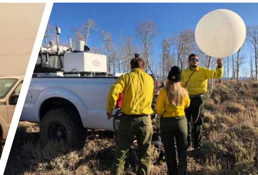
Lidar and radiosonde system deployed during the King fire in 2014.
