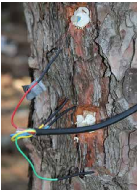
Evangelia Korakaki prepares the necessary equipment before the implementation of a planned field prescribed burn experiment in pine litter to monitor, measure, and record sap flow. Photos by Georgios Mantakas and Stavros Sofronas.
