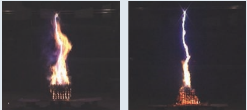
Photos show the breakdown flashes induced by the flame (left) or the plume (right) during small-scale experiments at SKLFS.
