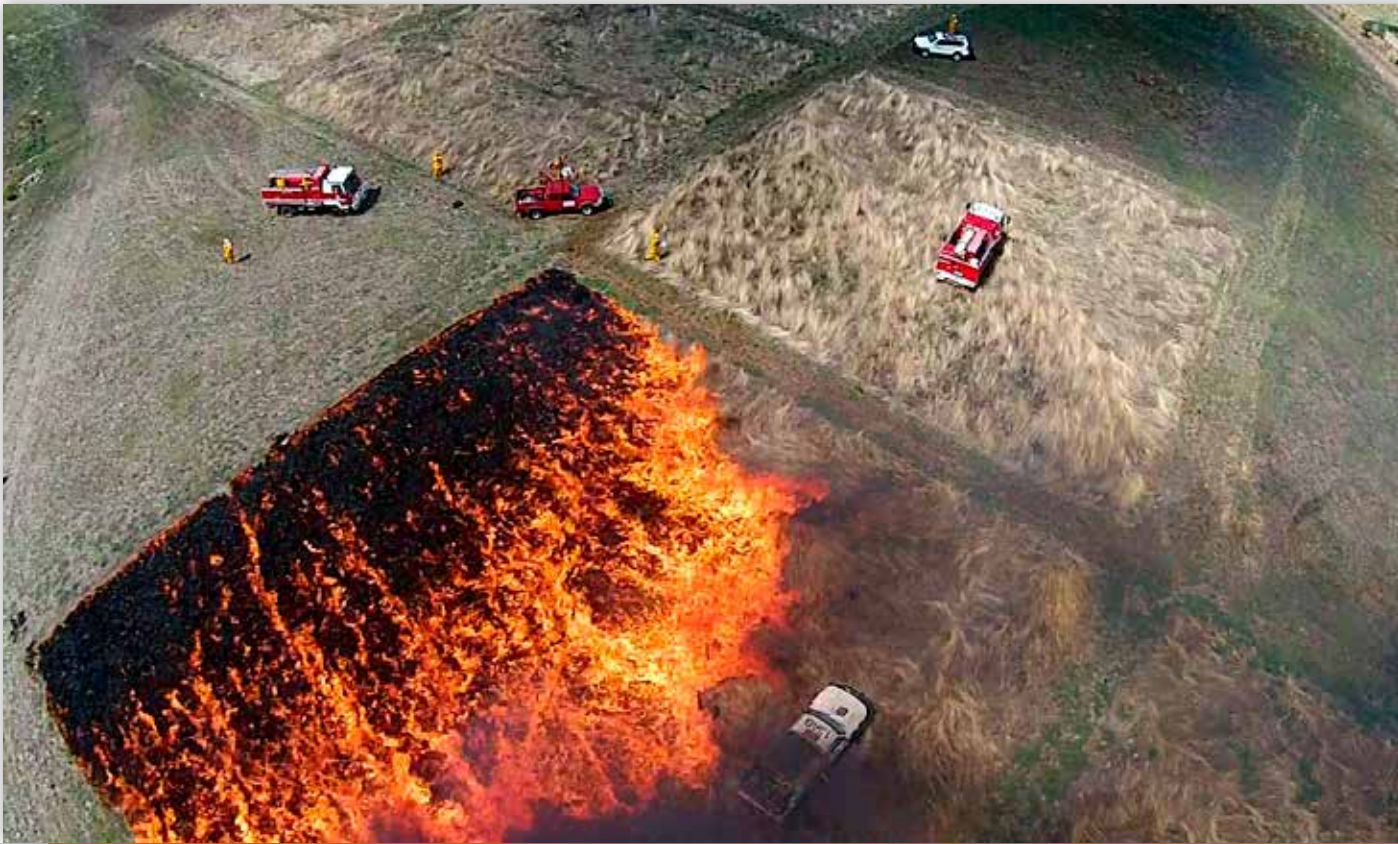
Wangaratta, Victoria -- an experimental grassland fire tests the flame-front impact on an ultra-light gel protected tanker vehicle. More on page 28 -- "Developing a Tanker Crew Protection System."
