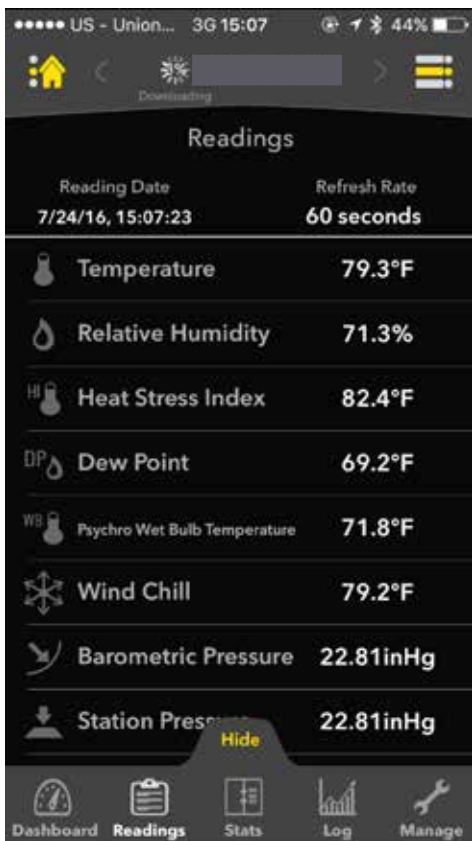
Screen shot from the Bluetooth real-time data link from the Kestrel 5500 to a smart phone
