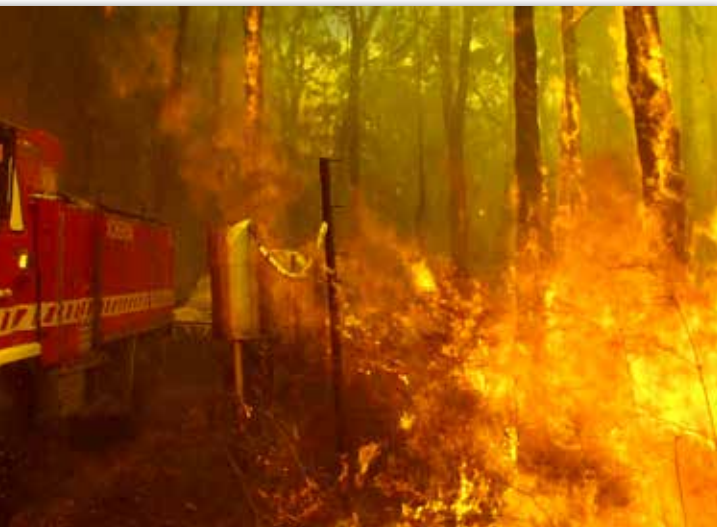
Figure 3. Brucknell, Victoria experimental bushfire pre-fire flame front impact on medium and ultra light fire fighting tankers.
