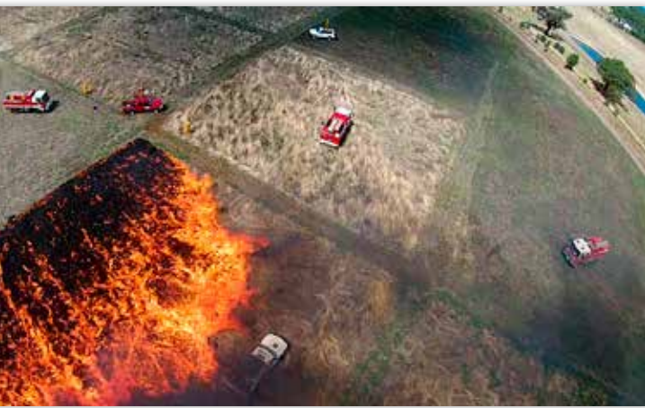
Figure 2. Wangaratta, Victoria grassland fire experimental test flame front impact on ultra-light gel protected tanker test vehicle.
