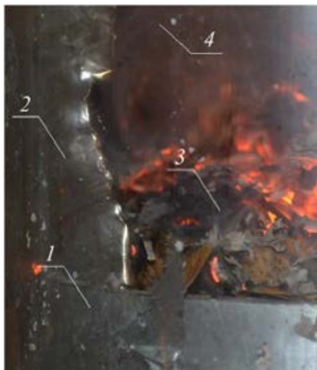
Fig. 4. Typical videogram of experiment with the suppression of thermal decomposition reaction of FFM (birch leaves) by the vapor-water mixture: 1 – metal sublayer; 2 – hollow cylinder; 3 – forest fuel material; 4 – vapor-water mixture.
