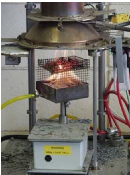
Fig.2. Experimental setup (from bottom to top): load cell, methane burner, incoming methane flame, wire-mesh sample holder, burning live fuel sample, outgoing flame (methane flame with the burning sample within the flame)
