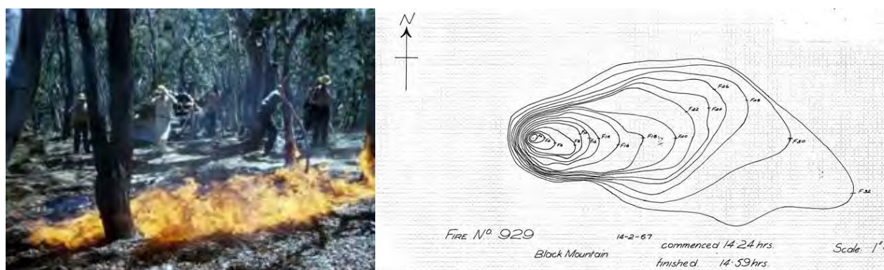
Figure 1. Experimental fire 929 in dry eucalypt forest at Black Mountain, ACT (left) and the fire isochrones represents the fire perimeter at 2-minute intervals (right).
