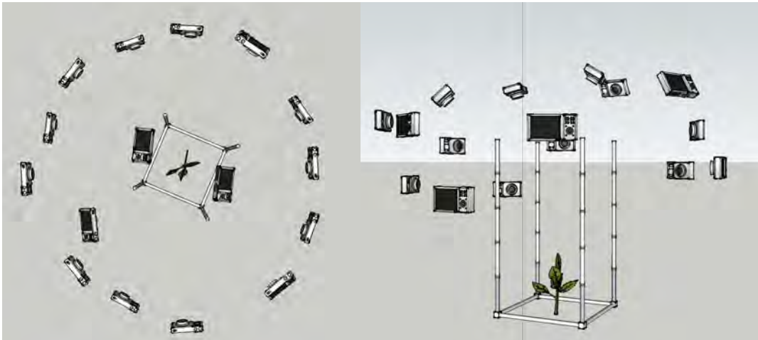
Figure 2: An simulated example of how images can be collected to provide strong geometry for 3D reconstruction of the scene. The figure also shows an example of a scaling quadrat.
