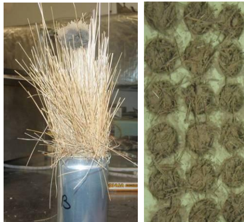
Fig. 8. A tussock sample with a disk placed on top (left), and organic embers in moulds (right).
