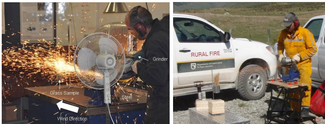
Fig. 6. Metal sparks experimental set-up in the laboratory (left) and the field (right).
