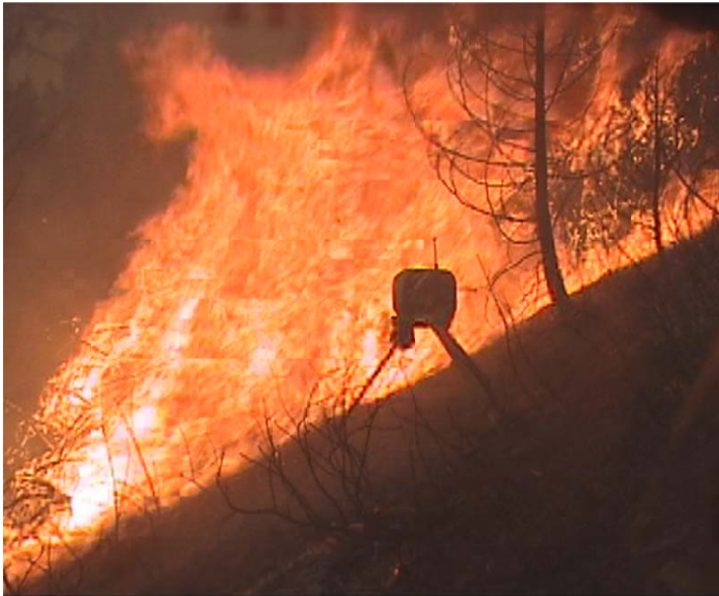
Fig.3-- Insitu Video Camera mounted on tripod in wildland fire.
