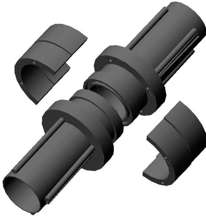
Fig. 3. Proposed hose coupler design
