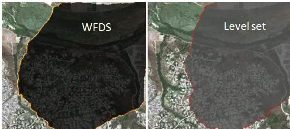
Fig. 11: Simulation of firespread over a 2 km x 2 km region with complex terrain encompassing a southern California community. The terrain was obtained from LiDAR data. For simplicity, and as a first step in model testing, the entire domain is covered in grass (image showing the roads, structures, and vegetation is used for ease of reference when comparing the figures). The WFDS (level set) simulations required 41 million (2000) grid cells; 16 (1) processors; and were 400 times slower (5 times faster) than real time.
