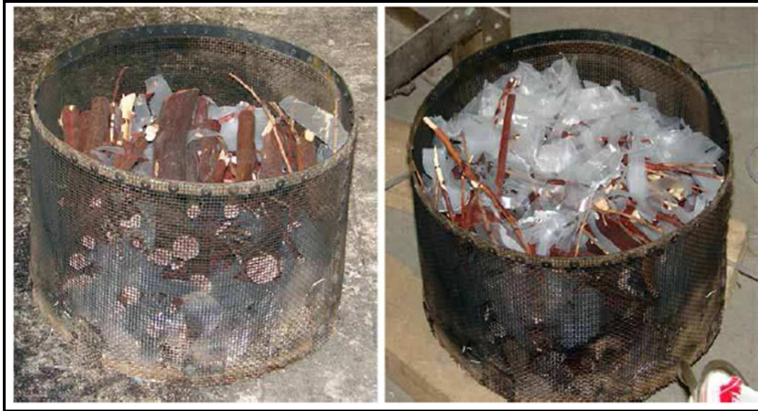
Fig. 1. Mixtures of clear polyethylene plastic (LDPE) and manzanita wood used to simulate debris piles containing 0.5% and 5.0% LDPE by mass.
