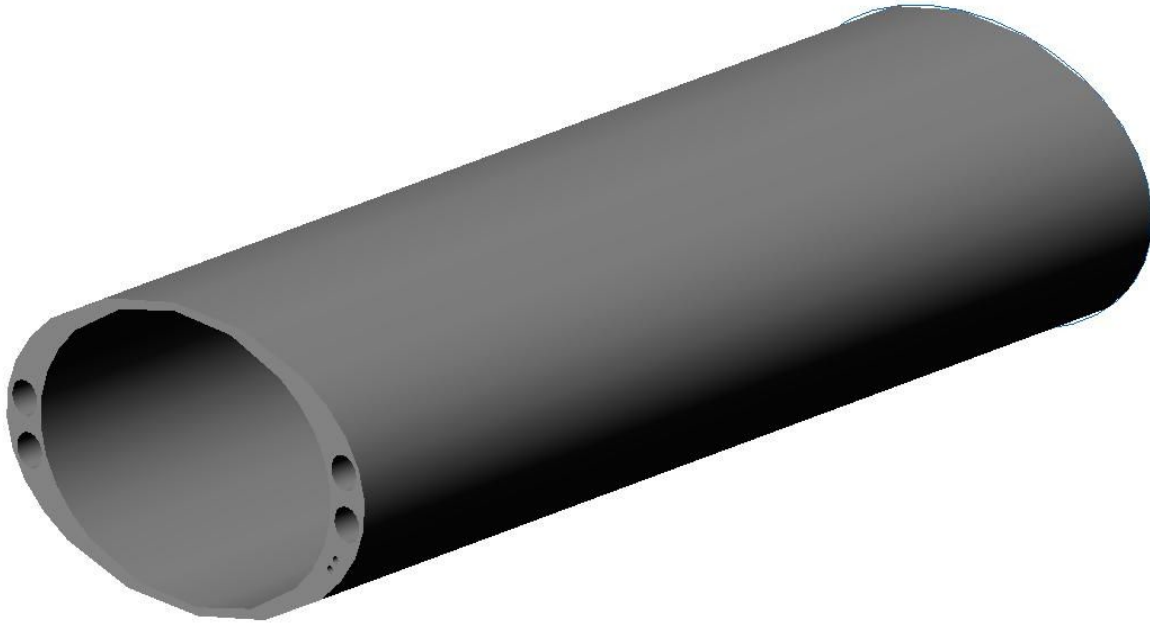
Fig. 2. Cross section of hose showing tunnels for attached wires.
