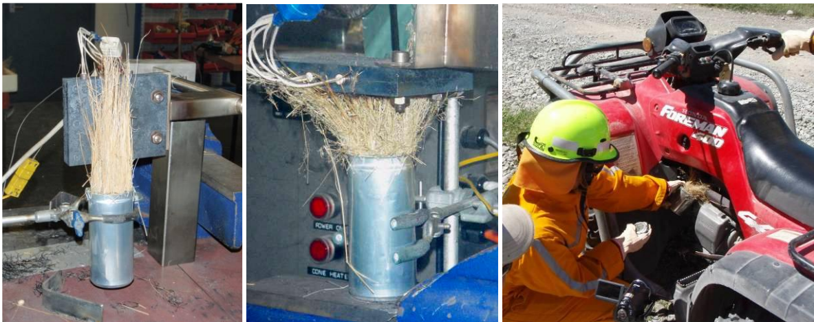
Fig. 2. Grass sample held in contact with the copper hot plate in vertical orientation (left) and horizontal orientation (middle), and field testing of a sample at the manifold of the ATV (right).
