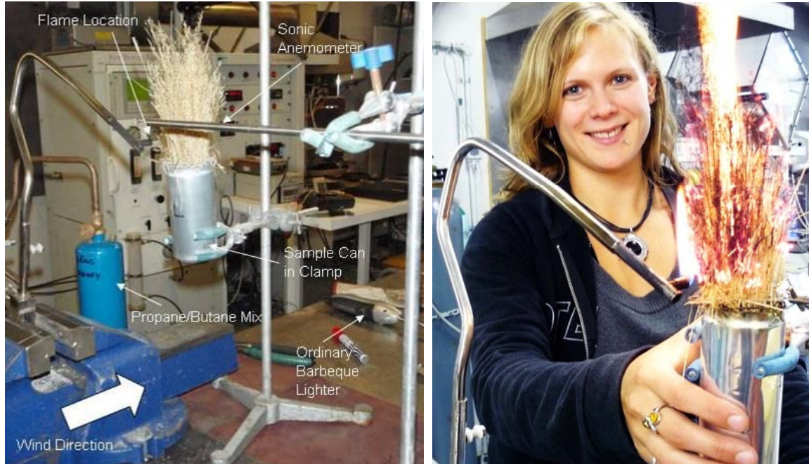
Fig. 9. Open flame experimental set-up (left) and H. Wakelin with a burning sample (right).
