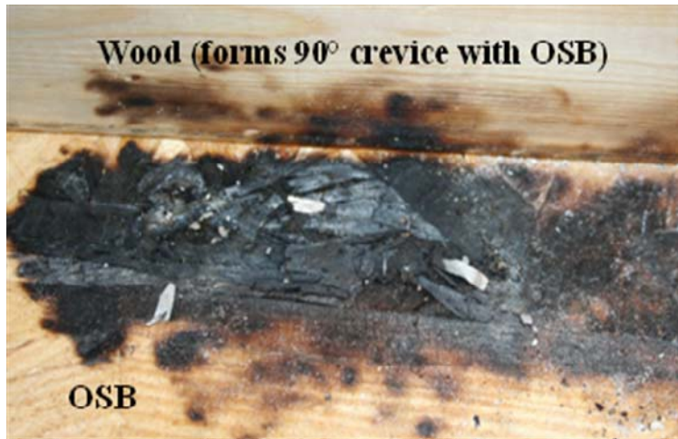
Figure 14 Images obtained (top view) for crevice filled with paper tests using 10 x 10 (2.0 mm) mesh using NIST Dragon’s LAIR.
