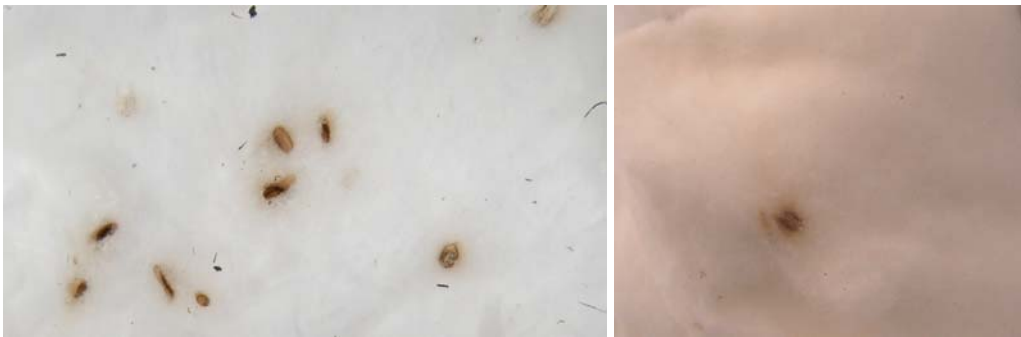
Figure 9 Images obtained for cotton tests using 4 by 4 (5.72 mm) mesh. The image on the right demonstrates complete burn through of the cotton.
