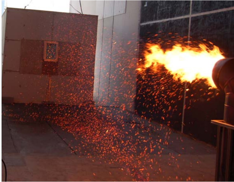
Figure 7 Typical experiment using NIST Firebrand Generator at BRI's FRWTF. The mesh installed in this experiment was 20 x 20 (1.04 mm), the wind tunnel speed was 7 m/s, and the Firebrand Generator was located 7.5 m from the structure.
