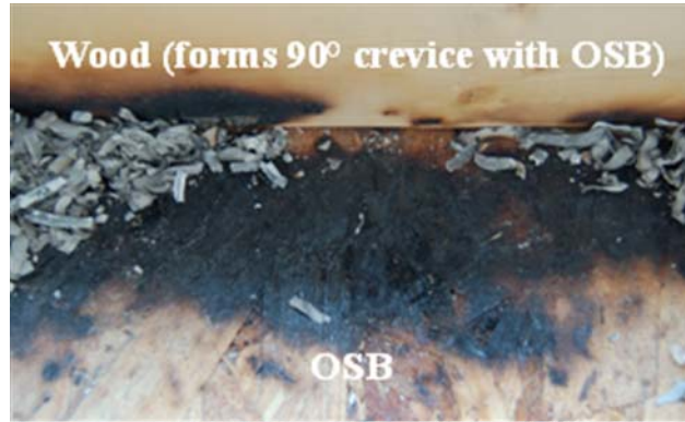
Figure 10 Images obtained (top view) for crevice filled with paper tests using 10 x 10 (2.0 mm) mesh.
